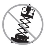
Do not raise the platform unless the machine is on a firm, level surface.
