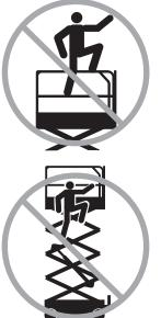
Do not sit, stand or climb on the platform guard rails. Maintain a firm footing on the platform floor at all times.
