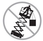
Do not place or attach fixed or overhanging loads to any part of this machine.
